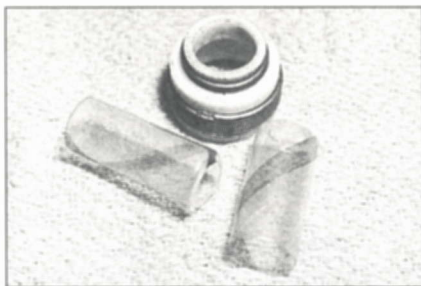
Protector tubes help ensure that the inside surface of the valve stem seal is not marred during installation.
