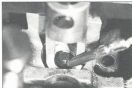
While depressing the retainer with the lever, fish out the keepers with the magnetic wand.
