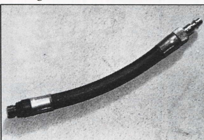
An adaptor such as this is needed to supply compressed air to prevent the valves from falling into the cylinder after you remove the valve springs.
