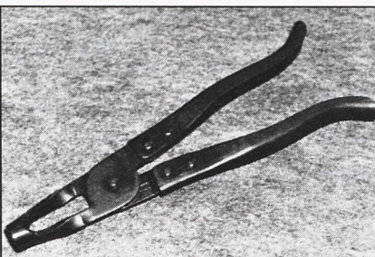
These special seal removers are just about the only way to reach the valve stem seals on 924s, Volkswagens and Audis.
