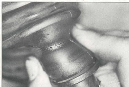
Here's an example of a boot that is soon to fail. Replacing and repacking the boot is much easier and cheaper than buying a new one.
